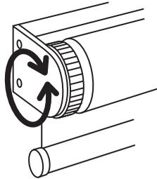
To adjust the spring tension on the roller, simply rotate the dial on the left side of the shade. Rotate the dial towards the floor to tighten (makes shade roll faster) or rotate towards the ceiling to loosen (makes shade roll slower).
